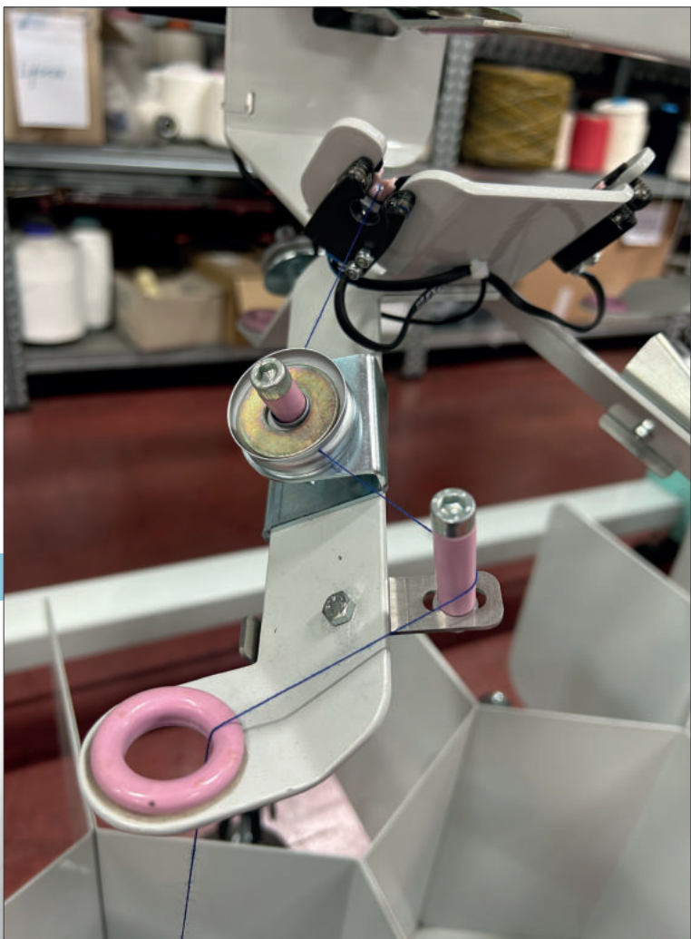
yarn tensioner for each single ply installed on the anti-ballon
